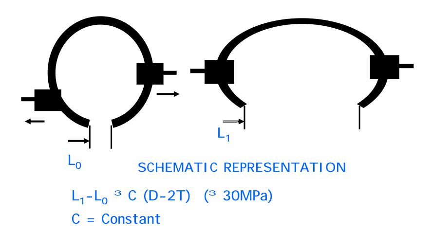
But exfoliation test is not a completely reliable method for checking bond strength. Hence twist fatigue test was developed
