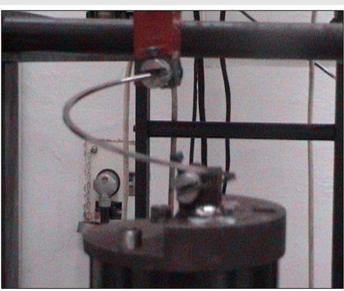
The free gap ends are clamped and one gap end will be pulled to the constant magnitude at the fixed frequency.
